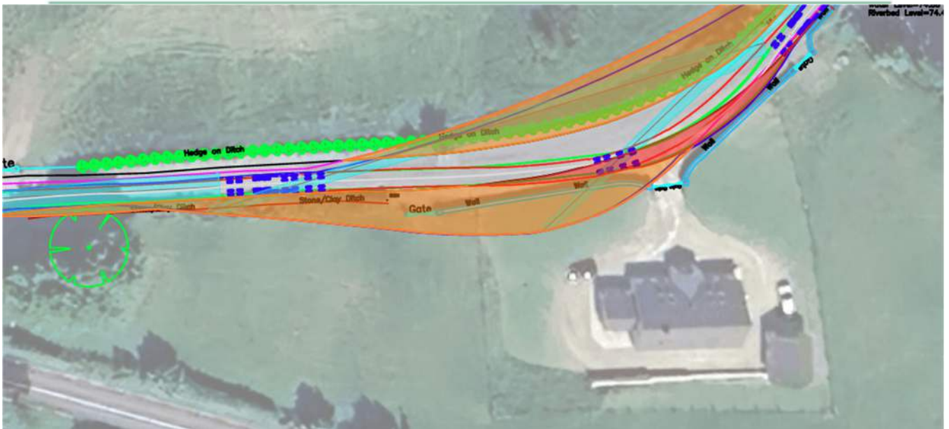
Figure 12: Extract from Location 01, Appendix 2.1 Turbine Delivery Route
